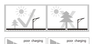
$\star$  Please choose a place where is full of sunlight and can be completely exposed to the sun, Notice that the solar panels must not be covered ,and must be exposed to the sun.
